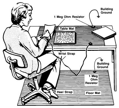
Figure 2. Static Safe Workstation
